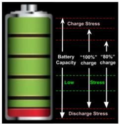
The life of a battery is reduced when at extreme high or low levels of charge<sup>46</sup>. To avoid cars reaching either end, not all of the battery capacity is made available.
